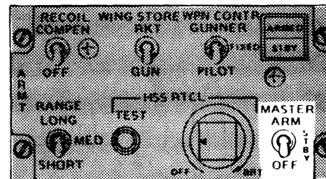
PILOT ARMT CONTROL PANEL
