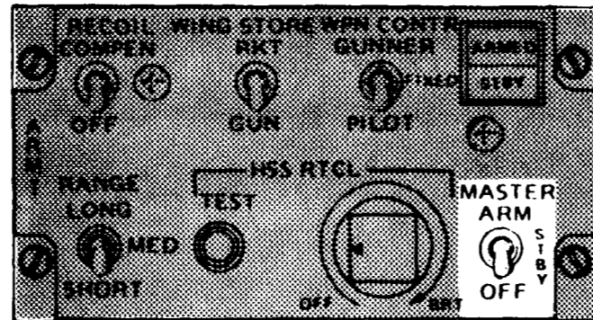
PILOT ARMT CONTROL PANEL
