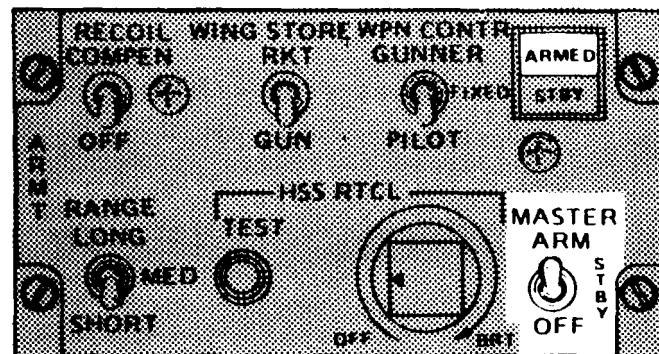
PILOT ARMT CONTROL PANEL
