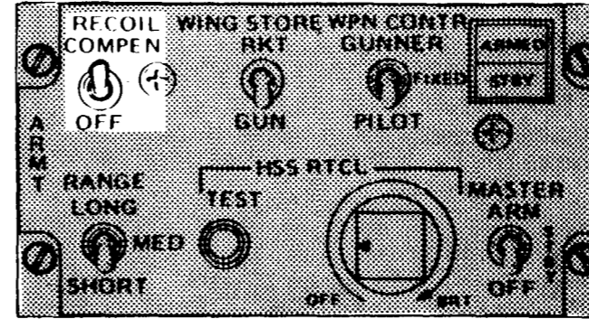
PILOT ARMT CONTROL PANEL
